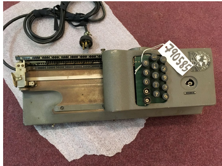
Remington Rand card punch machine, ca 1960. Card punch machine for punching holes in computer punch cards. In artifact collection storage at Ingenium. Photo credit: Jennifer Thivierge.
