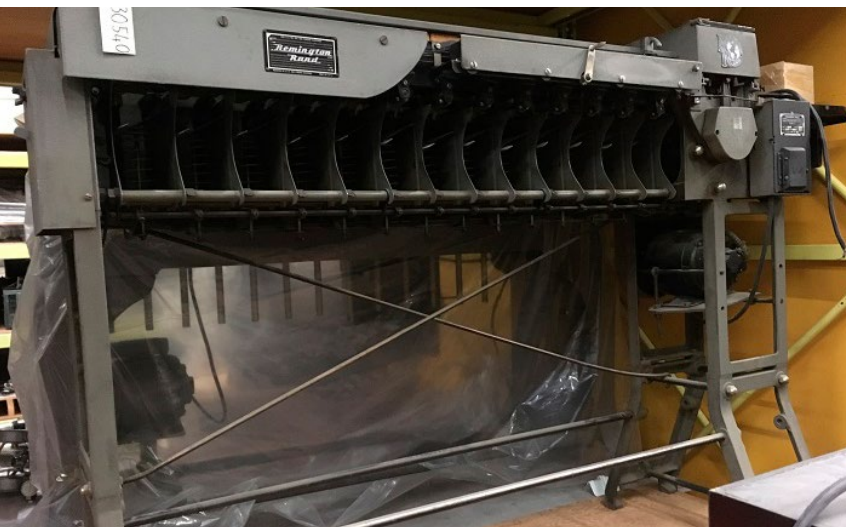
Remington Rand computer punch card sorting machine. In artifact collection storage at Ingenium. Photo credit: Ingenium.
